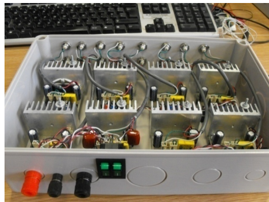
Figure 3.19 Power amplifier module.
