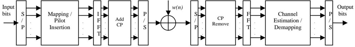
Figure 1. Block diagram of an optical OFDM.
