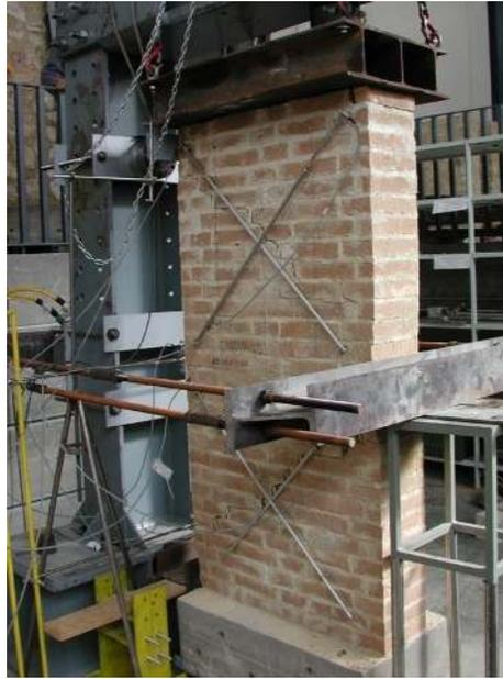
Fig. 3 Typical layout of a shear-compression test.
