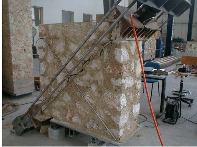
Fig. 1 Typical layout of a diagonal compression test.
