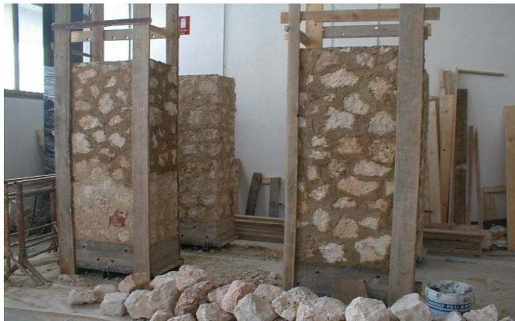
Fig. 4 Diagonal compression and shear-compression tests carried out on mortar small-scale panels.
