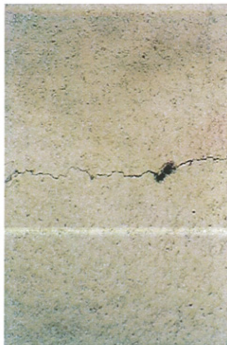
Figure 6.42 Optical micrograph of crack growth. Crack was 2.3 mm length
