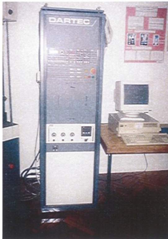
Figure 5.2 A Dartec series M9000 controller that is used in conjunction with the Mayes dynamic testing machine.
