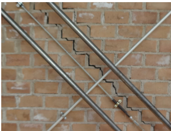
Fig. 5 Detail of failure (unreinforced panel)
