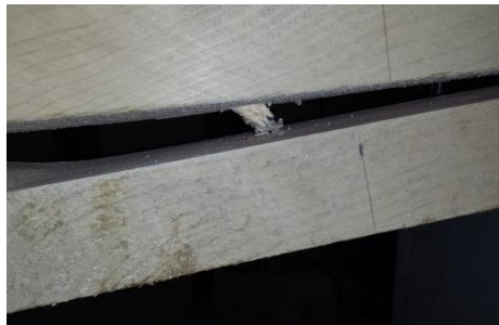
Figure 8. Pull out of the BFRP spike.
