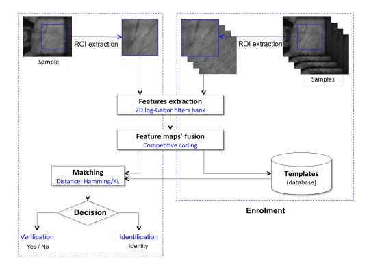
Figure 1: Multi-spectral palmprint recognition process flow diagram.
