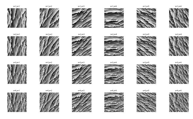
Figure 3: An example of filtered images along four scales and six orientations obtained using the bank of 24 log-Gabor filters applied on a ROI image under Green spectral band.
