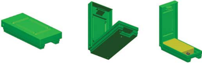
Fig. 9. Modeled AP landmine PMA-1. Green is plastic ( \epsilon = 2.5 ), gray is perfect conductor (PEC), and yellow is rubber ( \epsilon = 6 ).
