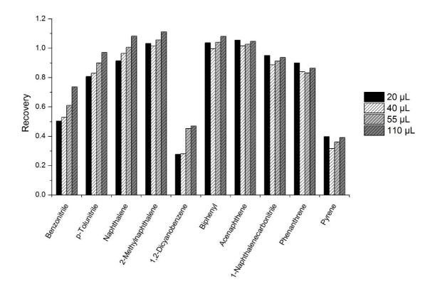
Figure 3 – Observed recovery for select compounds after HSSE extraction of spiked blank cartridges with stir bars of different coating volumes.
