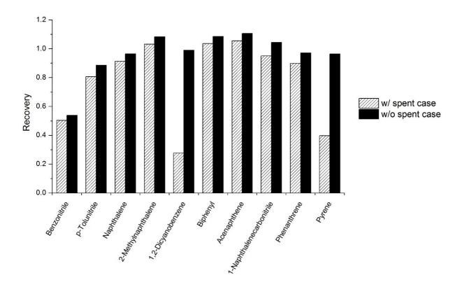
Figure 6 – Difference in recovery of target analytes in the presence ("w/") and absence ("w/o") of blank cartridges.
