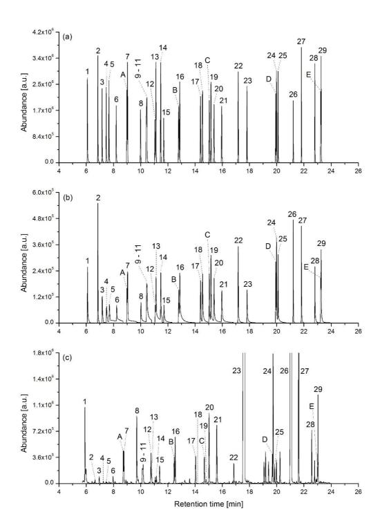
**Figure 1**– Examples of chromatograms for (a) the direct injection of liquid standards with the optimised separation method, (b) the impact on the GC performances after analysis of 37 real samples spiked with 10  $\mu$ L of dichloromethane, and (c) a 9 mm spent cartridge from Geco, analysed after 1 h of ageing. Correspondence between numbers and peaks is explained in Table 1.
