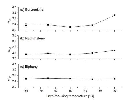
Figure 5 – Plot of peak widths at half height  $(w_{1/2})$  for select 3 target analytes as a function of cryo-focusing temperature.
