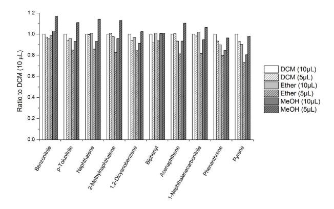
Figure 2 – Observed response for select compounds after HSSE extraction of samples spiked with different carrier solvents and volumes. For the sake of comparison, values are normalised by those observed using 10  $\mu$ L of dichloromethane (DCM). Values for deuterated compounds were very similar to their non-deuterated analogues (not shown here).
