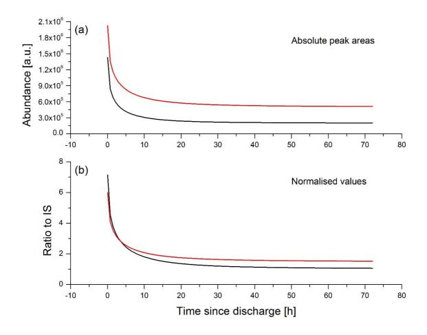
**Figure 8** – Comparison of two ageing curves for pyrene taken at 3 months interval (a) without normalisation and (b) with normalisation to the corresponding deuterated standard (pyrene-d10).
