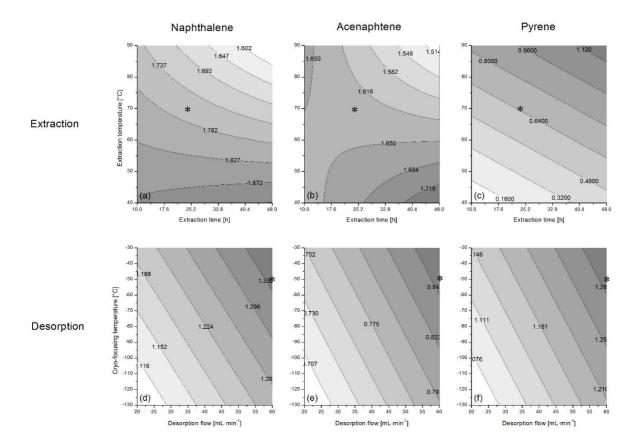
**Figure 4** – Evaluated surface response for select compounds and particularly influent parameters in the optimisation of both, the extraction (a-c) and desorption conditions (d-f). An asterisk (\*) indicates the chosen optimal conditions. Complete illustrations for all the compounds involved in optimisation are reported in Electronic Supporting Material.
