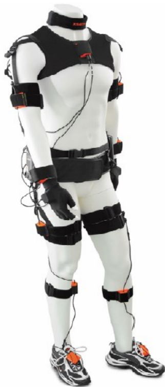
Figure 4-6 Photograph from XSens MVN user manual (2012) showing tracker and neoprene band locations
