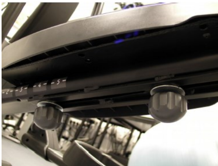
Figure 3-2 A close up view of the adjustable footplate (image from FRED operating instructions)
