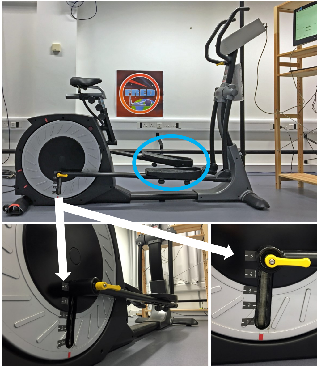
Figure 3-1 The FRED with the adjustable crank highlighted by white arrows the footplates shown in the blue circle
