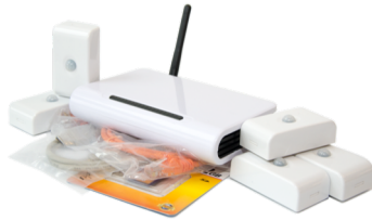
Figure 1: BuildAX sensor toolkit comprising of a base unit and low-cost sensor nodes, which sample temperature, humidity, light, movement and magnetic switch (for doors and windows).
