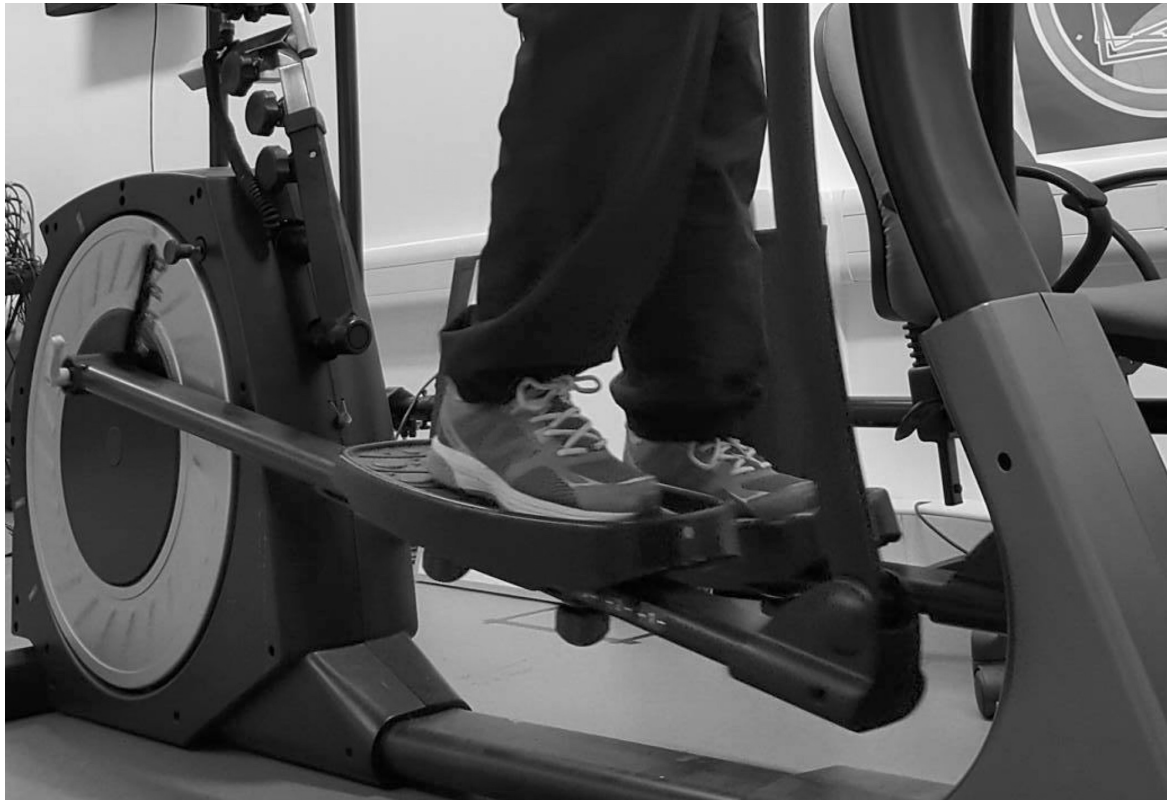
Fig. 6.1 Functional Readaptive Exercise Device (FRED): a modified cross trainer which offers minimal resistance requiring smooth control to recruit muscles in the lower back and abdomen.
