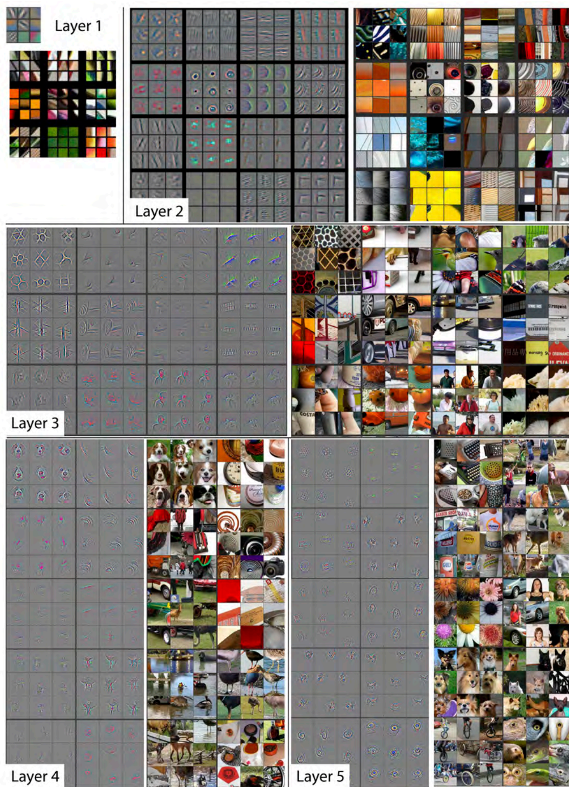
Figure 2.7: Convolutional Feature Filter Examples: (Layer 1) - Generic edges, (Layer 2) - Generic lines and curves, (Layer 3, 4, 5) - Domain specific shapes.
