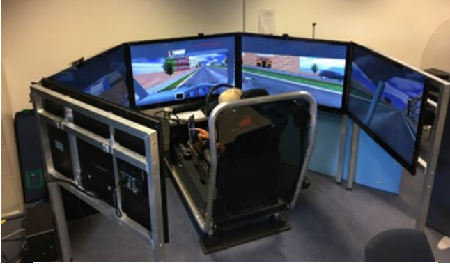
Fig. 1. Fixed-based ST Software Jentig50 driving simulator
