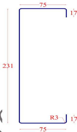
Figure 11: Benchmark LCB section
