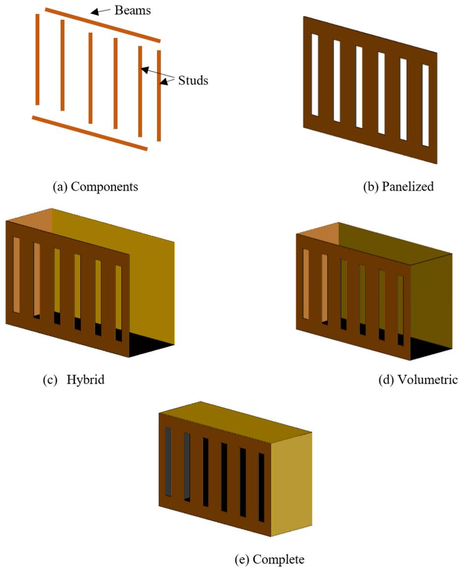
Figure 3: Typologies of off-site construction method
