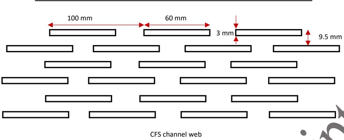
Figure 18: Slots configuration and dimensions
