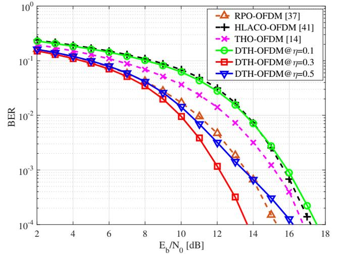
Fig. 7. BER comparisons between the proposed DTH-OFDM with various dimming level  $\eta$  and the RPO-OFDM, HLACO-OFDM with 3 layers and THO-OFDM, where the modulation formats for ACO-OFDM and PAM-DMT are set as 16QAM and 4PAM.
