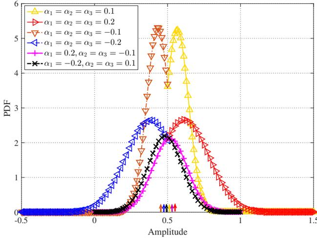
Fig. 3. PDFs of DTH-OFDM with various dimming factors  $\alpha_i$  when  $I_{\text{bias}} = 0.5$ , where six different colours arrows all represent the Dirac delta function in the point of  $I_{\text{bias}}$ .
