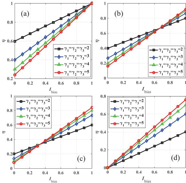
Fig. 6. The dimming level  $\eta$  as a function of  $I_{\text{bias}}$  with various scaling factors  $\gamma_i$  in DTH-OFDM. (a) Dimming factors  $\alpha_i > 0$ ; (b) Dimming factors  $\alpha_1, \alpha_2 > 0, \alpha_3 < 0$ ; (c) Dimming factors  $\alpha_1 > 0, \alpha_2, \alpha_3 < 0$ ; (d) Dimming factors  $\alpha_i < 0$ .
