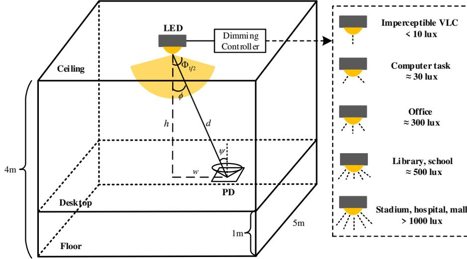
Fig. 1. Channel geometric model for indoor VLC systems.
