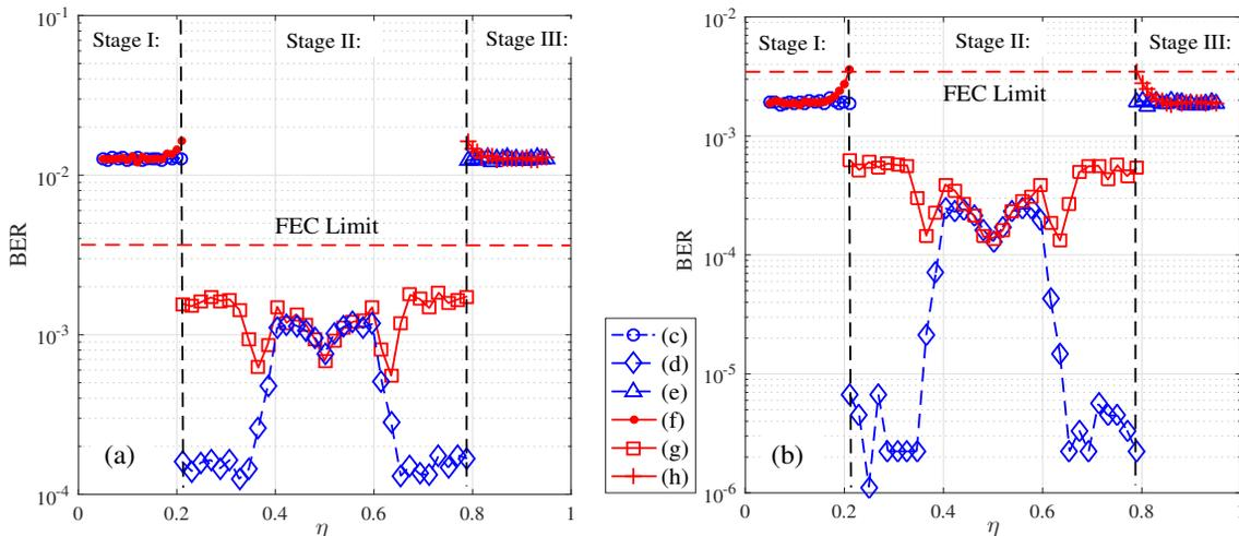
Fig. 8. BER performance of the proposed DTH-OFDM as a function of  $\eta$  using 16QAM and 4PAM when (a)  $\frac{E_b}{N_0} = 14$  dB and (b)  $\frac{E_b}{N_0} = 16$  dB, where (c)-(e) represent the different dimming stages without considering LED nonlinearity while (f)-(h) represent that considering LED nonlinearity.
