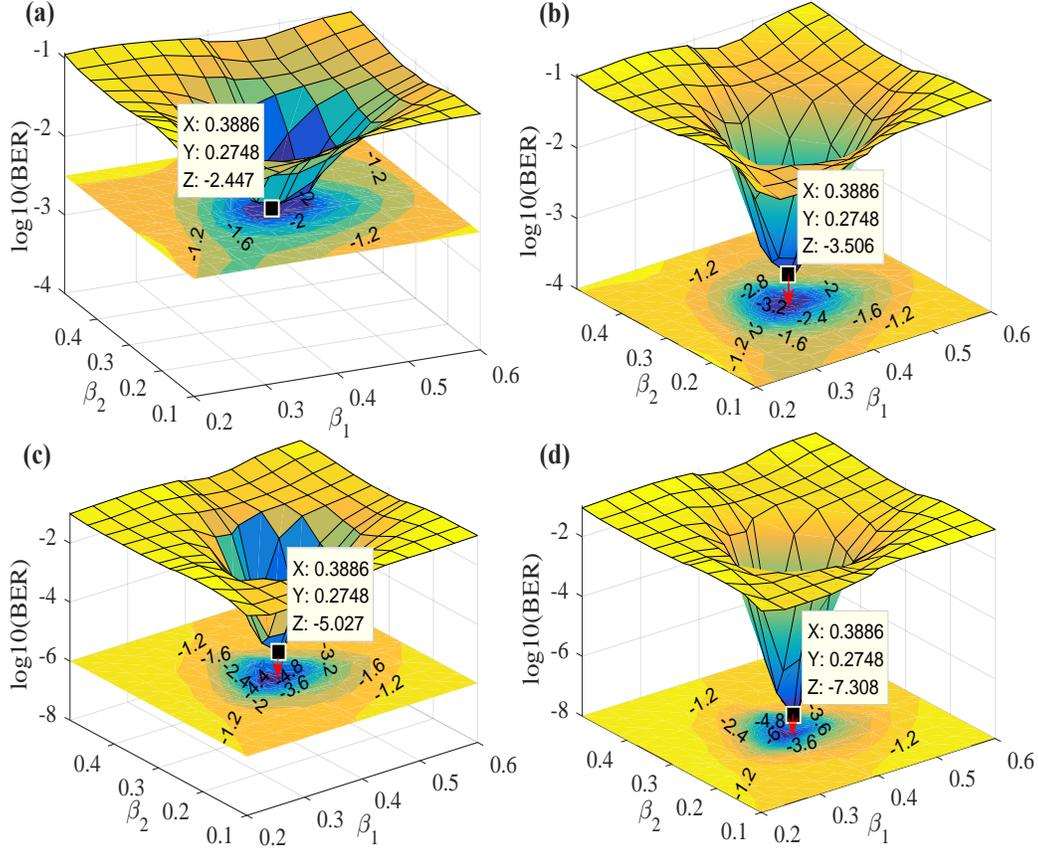
Fig. 5. BER performance of THO-OFDM and its contour map of the projection in X-O-Y plane v.s.  $\beta_1$  and  $\beta_2$  when using 16QAM and 4PAM, (a)  $\frac{E_b}{N_0} = 14$  dB, (b)  $\frac{E_b}{N_0} = 16$  dB, (c)  $\frac{E_b}{N_0} = 18$  dB and (d)  $\frac{E_b}{N_0} = 20$  dB.
