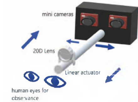
Fig. 1.3: The conceptual illustration of the proposed Head Mounted Device (HMD) for capturing retinal fundus images in [5]. Image reproduced from [5].
