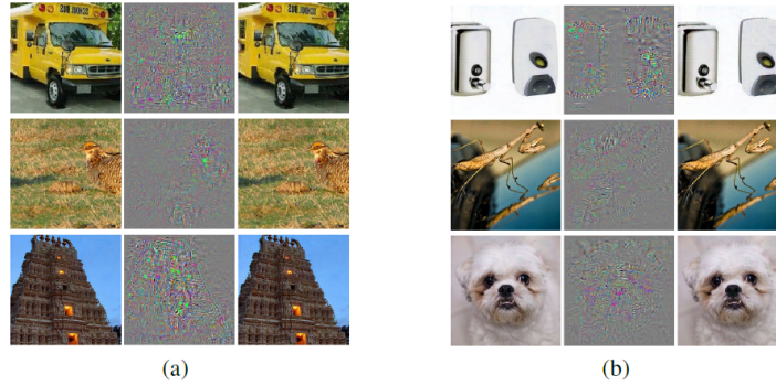
Fig. 1.17: An adversarial examples generated for AlexNet [20] using the method proposed in [34]. In each set of samples (a and b), the images on the left column are the original images while the right column contains the adversarial examples which lead to misclassification. The middle column illustrates the differences between the original image and the adversarial example magnified by 10 times. Image reproduced from [34].
