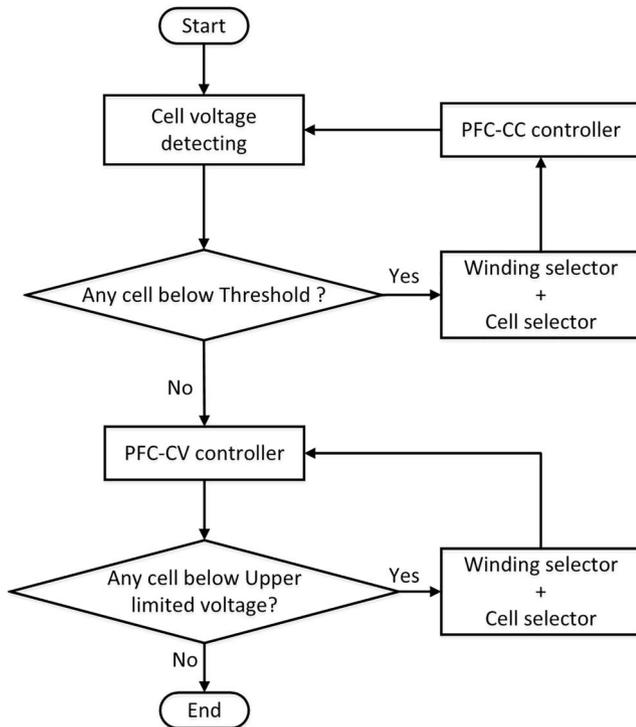
FIGURE 7 Flow chart of the proposed control algorithm
