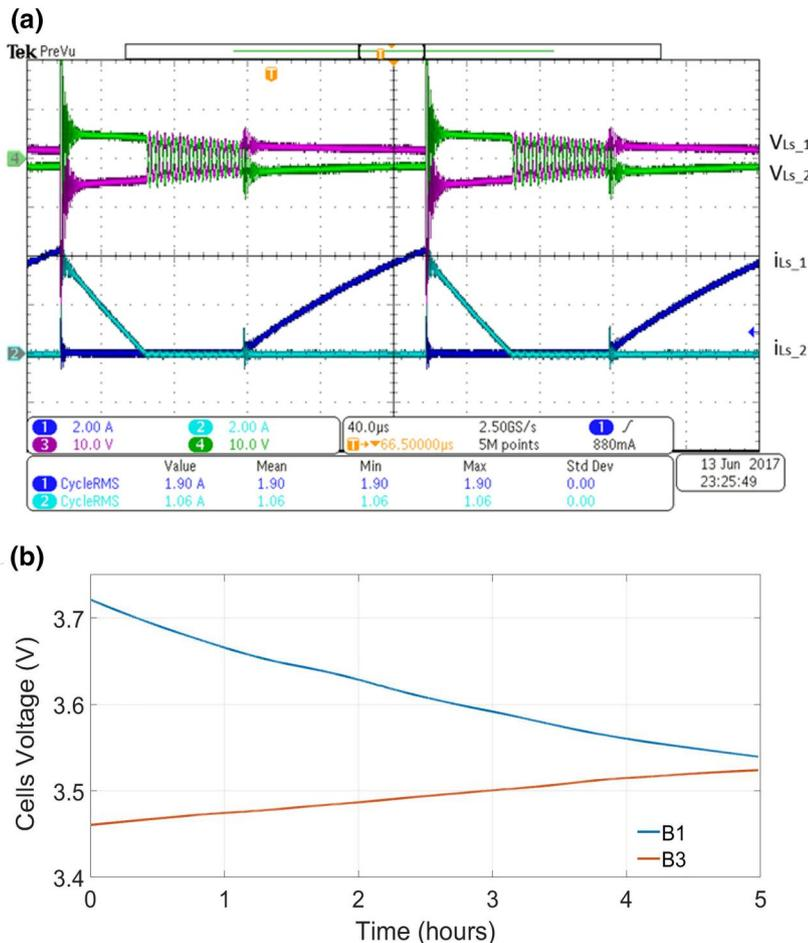
FIGURE 12 Waveforms of voltage equalisation from B<sub>1</sub> to B<sub>3</sub>: (a) voltage and current in the converter; (b) cells voltage
