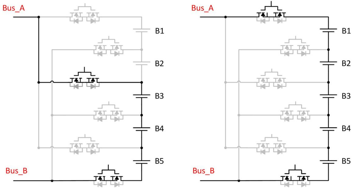
FIGURE 3 Examples of battery strings as sink cells
