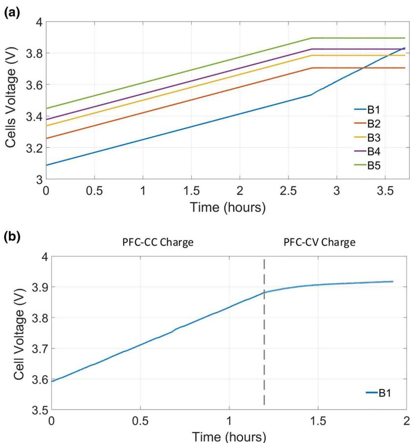
**FIGURE 11** Cells voltages during charging under (a) open-loop control; (b) power factor control-CC control
