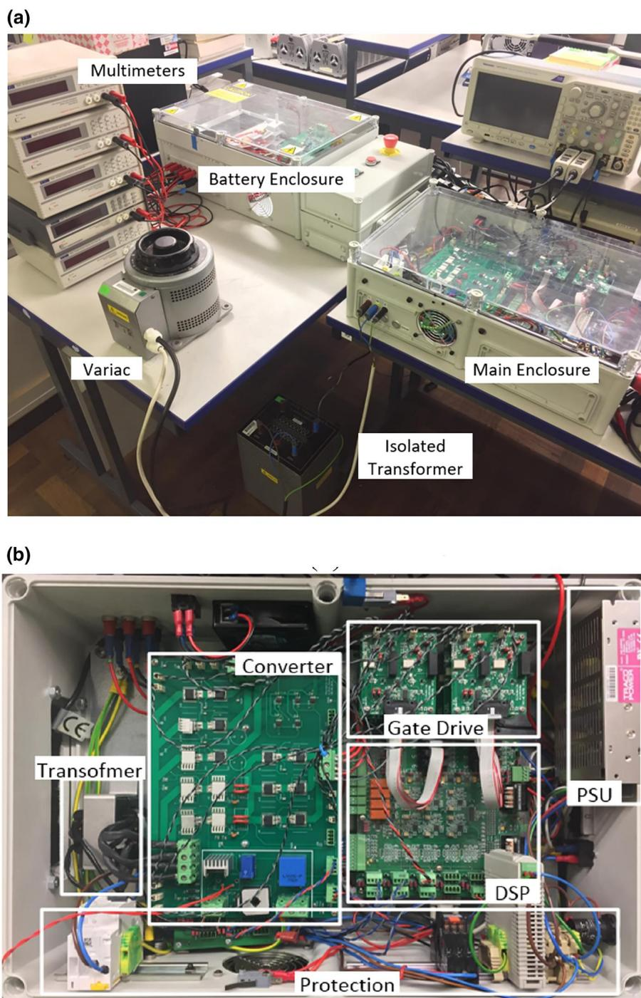
FIGURE 9 Photos (a) test bench; (b) prototype converter
