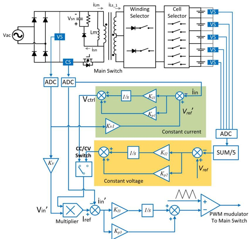
FIGURE 6 Diagram of the proposed circuit with the power factor control-CC-CV controller
