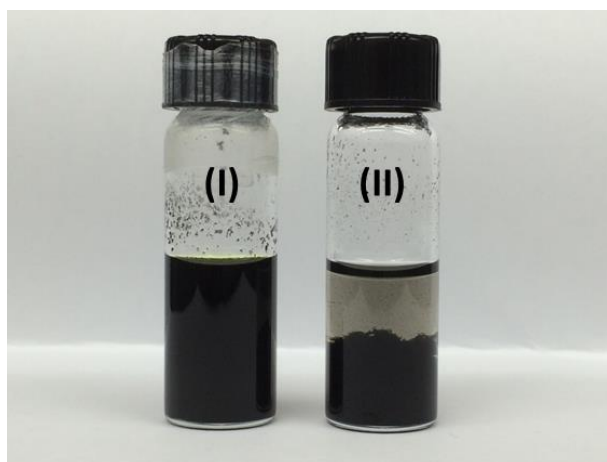
Figure S3. Digital photographs of (I) the \text{CH}_3\text{NH}_3\text{PbI}_{3-x}\text{Cl}_x/\text{SWNTs} precursor and (II) SWNTs in N, N-dimethylformamide (DMF) solutions taken 24 h after preparation. A homogeneous, dark dispersion of SWNTs in DMF solution of \text{CH}_3\text{NH}_3\text{I} and \text{PbCl}_2 was prepared, and remarkably, it remained stable for more than 24 h without precipitation, while the pristine SWNTs quickly precipitated out in DMF solution.
