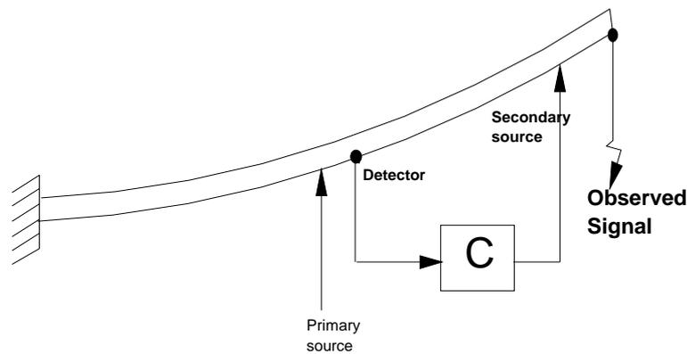
Figure 1. Active vibration control structure
