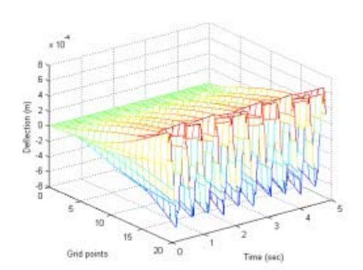
Figure 10. Beam fluctuation along its length before cancellation
