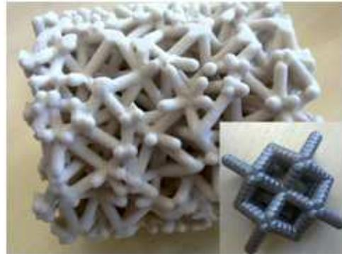
Figure 3: Randomised and regular (in inset) geometry structures
