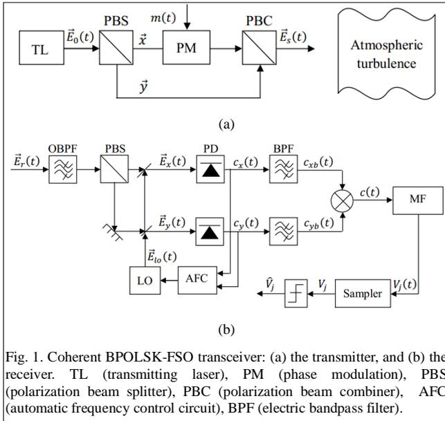
Fig. 1. Coherent BPOLSK-FSO transceiver: (a) the transmitter, and (b) the receiver. TL (transmitting laser), PM (phase modulation), PBS (polarization beam splitter), PBC (polarization beam combiner), AFC (automatic frequency control circuit), BPF (electric bandpass filter).
