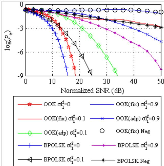
Fig. 2: Comparisons of BER performances of BPOLSK and OOK schemes against the normalized electric SNR  $E[\mathcal{R}P_r P_{lo}] = 1$  in the presence of turbulence.
