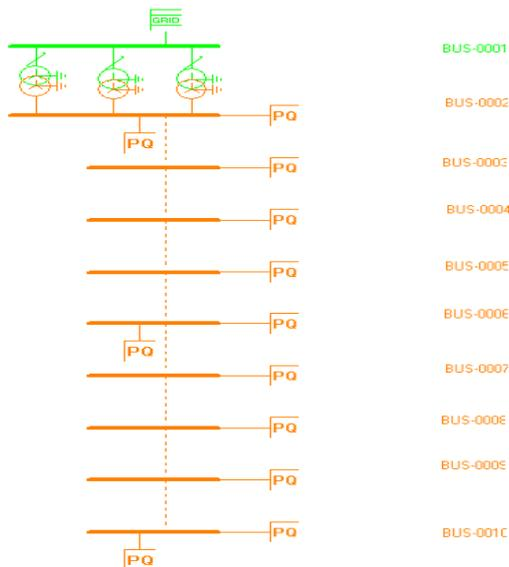
Figure 9. ERACS model of a 10 kV feeder, supplied by 35/10 kV 20 MVA transformers.
