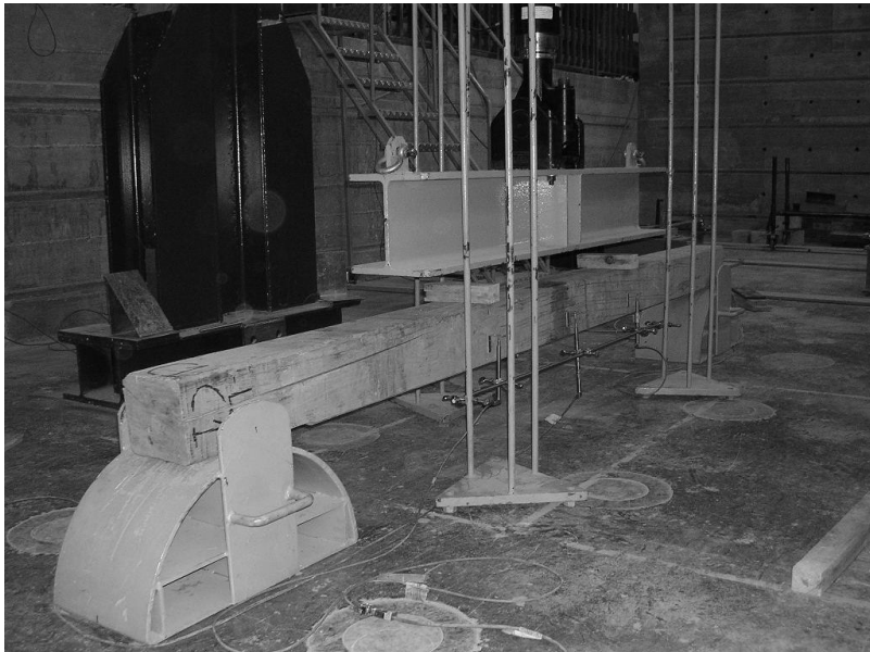
Figure 8. Flexural test set-up.
