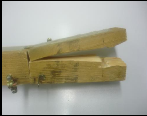
(b) Wood rupture.
