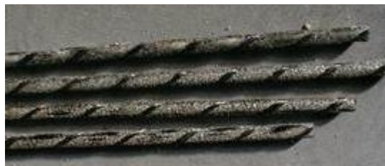
Figure 3. Carbon fibre-reinforced polymer (CFRP) bars: bars are sandblasted and superficially deformed.
