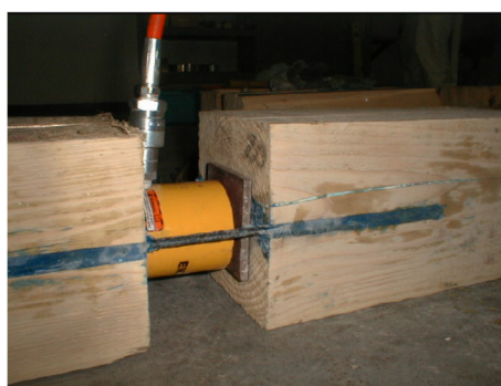
Figure 7. Pull-out test arrangement (tests without strain gauges).
