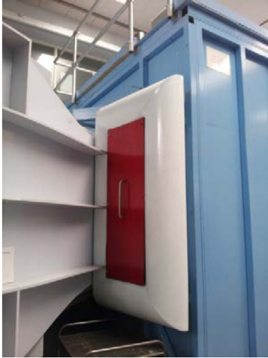
Figure 8. TGS Inlet trumpet sealed shut for conventional operation of wind tunnel without TGS.
