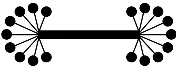
Fig. 6. Example of the grouping method. Edges are drawn from each node to a position slightly offset from the cluster's centroid. From here the edges are grouped and drawn to the centroid of the corresponding cluster where the group then splits apart again to make the individual connections.
