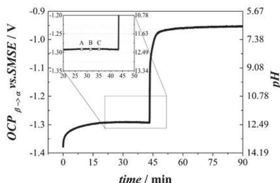
**Figure 1.** Potential transient (left axis) and corresponding pH (right axis) recorded with a 250  $\mu\text{m}$  diameter nano-structured PdH microelectrode during the carbonation of a saturated  $\text{Ca}(\text{OH})_2$  solution at 23°C and 0.167 atm  $p_{\text{CO}_2}$ .
