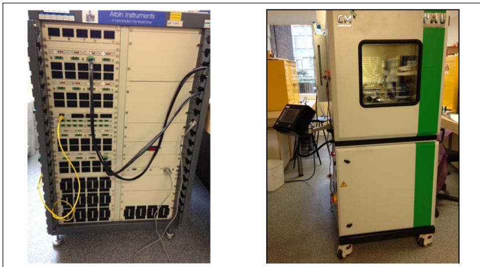
Figure 5: Lab arrangement: showing Arbin battery charger (left) and environment chamber (right)
