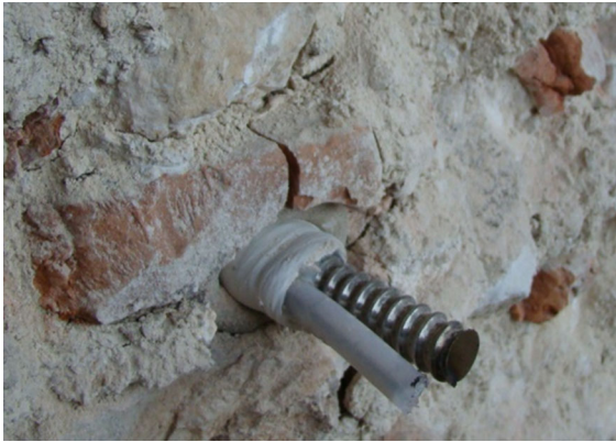
Fig. 6 Typical masonry failure mode during pull-out tests
