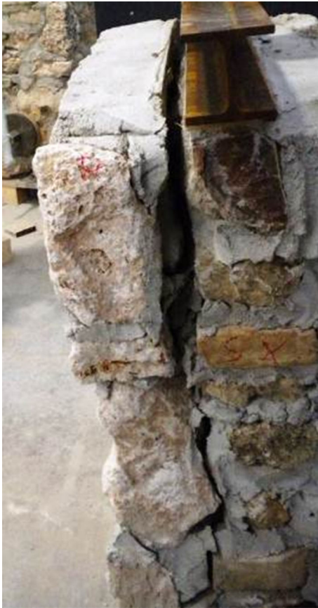
Fig. 7 Failure mode (unreinforced panel)
