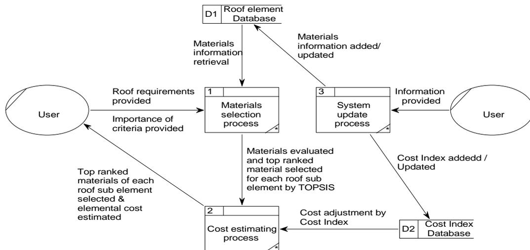
Figure 5: Level 1 data flow diagram of KDSMS
