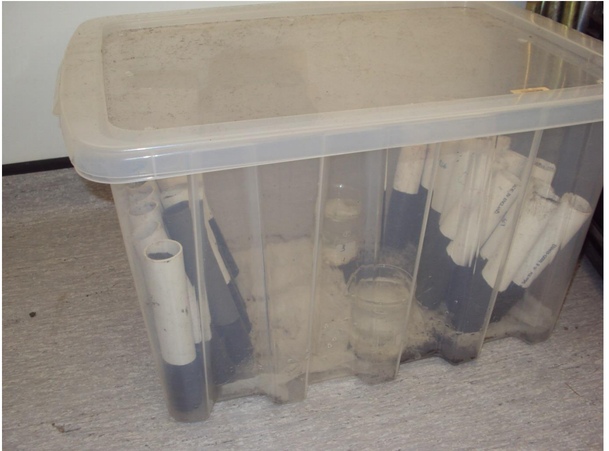
Figure 3.11: PVC microcosm storage box used during the pilot study of PAH bioremediation in soil
