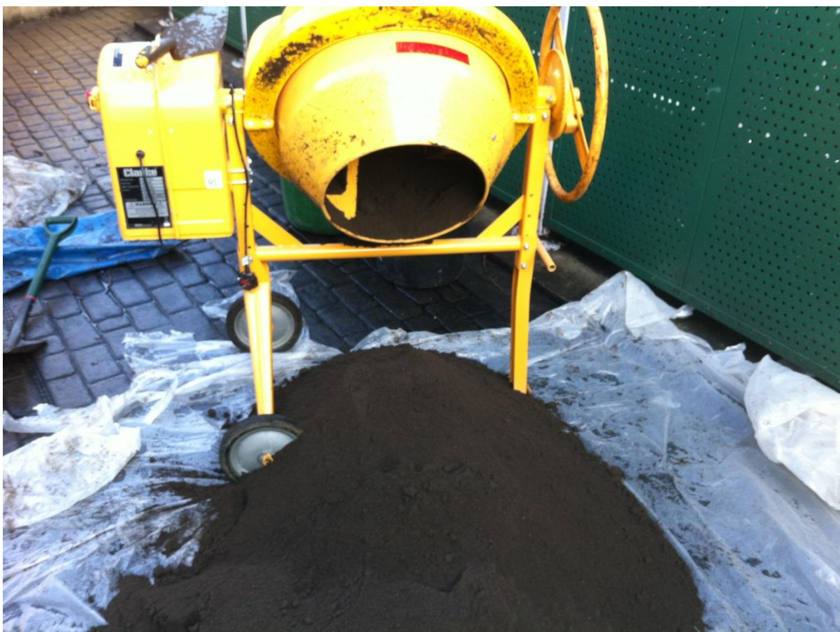
Figure 3.10: Soil spiking and mixing using an electric cement mixer
