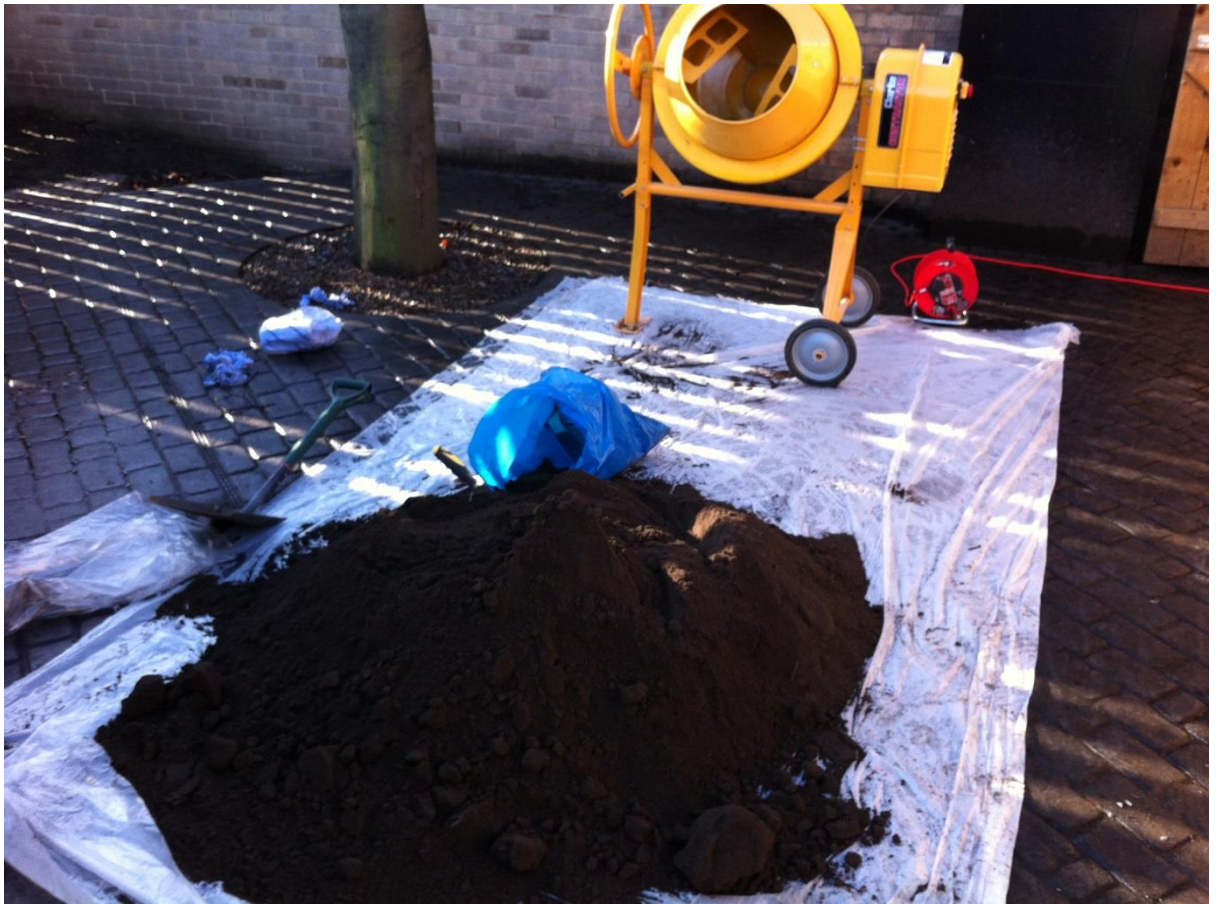
Figure 4.1: Soil spiking and mixing using an electric cement mixer
