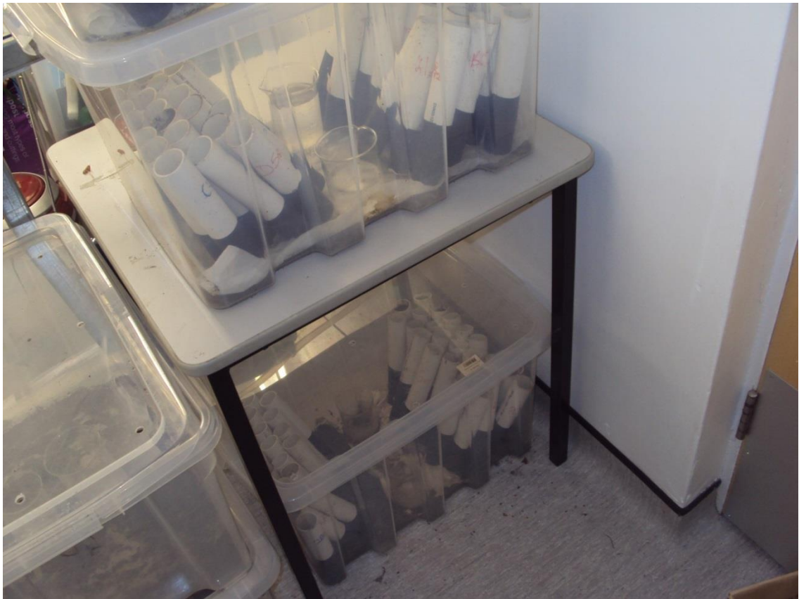
Figure 4.2: PVC microcosm storage box used during the main study of PAH bioremediation in soil
