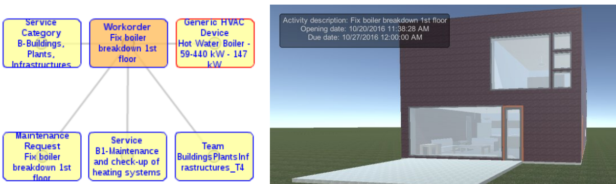
FIG. 11: Definition of a maintenance work order in Openmaint (left) and displaying maintenance work order data in Unity
