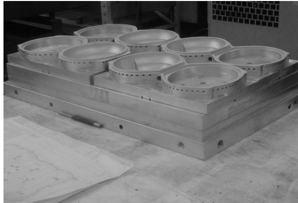
Figure 4: Multi – Cavity Mould Tool
