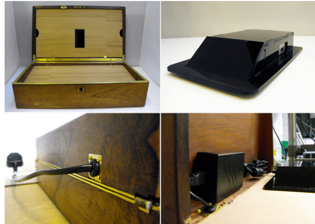
Figure 2. Clockwise from top left: Augmented writing box (open) refitted with wood panels and brass lining; 3D printed acrylic case for printer; Printer power supply hidden in upper panel; Power cord exiting rear of box through brass fixture.
