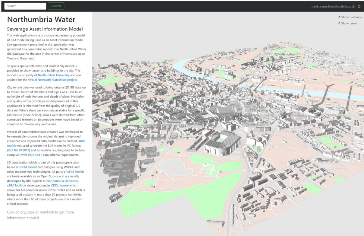
Fig. 10. Landing page of the SSAIM web application. The main part of the screen displays the three-dimensional city model and sewerage network, which can be explored using standard zoom features.
