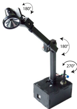
Figure 2. The lamp prototype for the first study with a potentiometer to control the light intensity.
