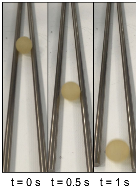
Figure 6.9: Analogy for V-Shaped channels: solid sphere suspended between two solid beams rolls towards the wider end.
