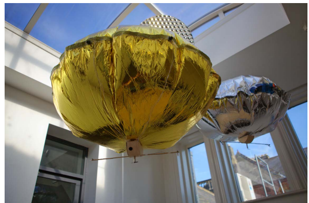
Figure 1. Diri #1 and Diri #2 (from the term Dirigibles, i.e. airships) - the autonomous helium balloons.
