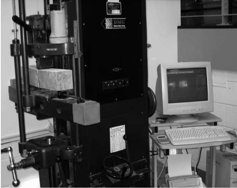
Figure 6 – Denison [DMG 67], beam sample and linked computer.
