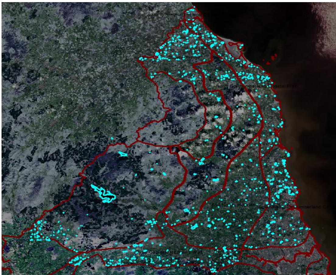
Figure A.6: Water bodies identified on Landsat-8 at 1:20,000 scale by land/water 5-6-4 band combination
