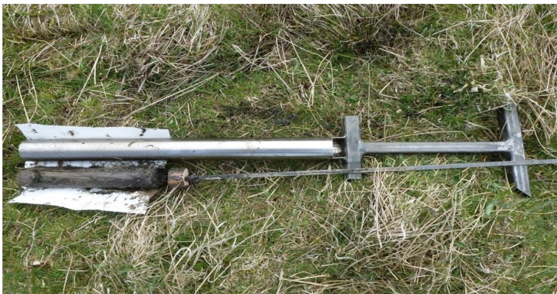
Figure B.1: Photo of the pole corer used to down core sediment collection at Druridge pools and a sediment core collected from a pond
