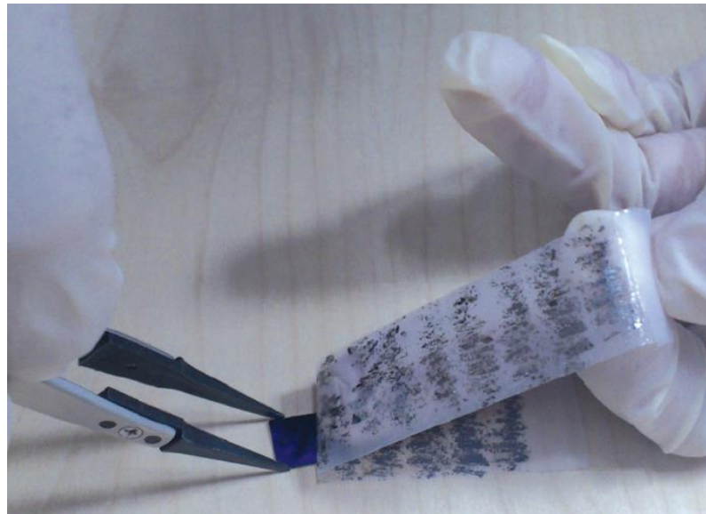
Figure 2. 4. Scotch tape method of graphene synthesis from graphite block [191].
