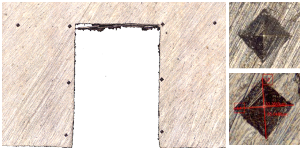
Figure 8.11: Hardness measurement using Alicona microscope.
