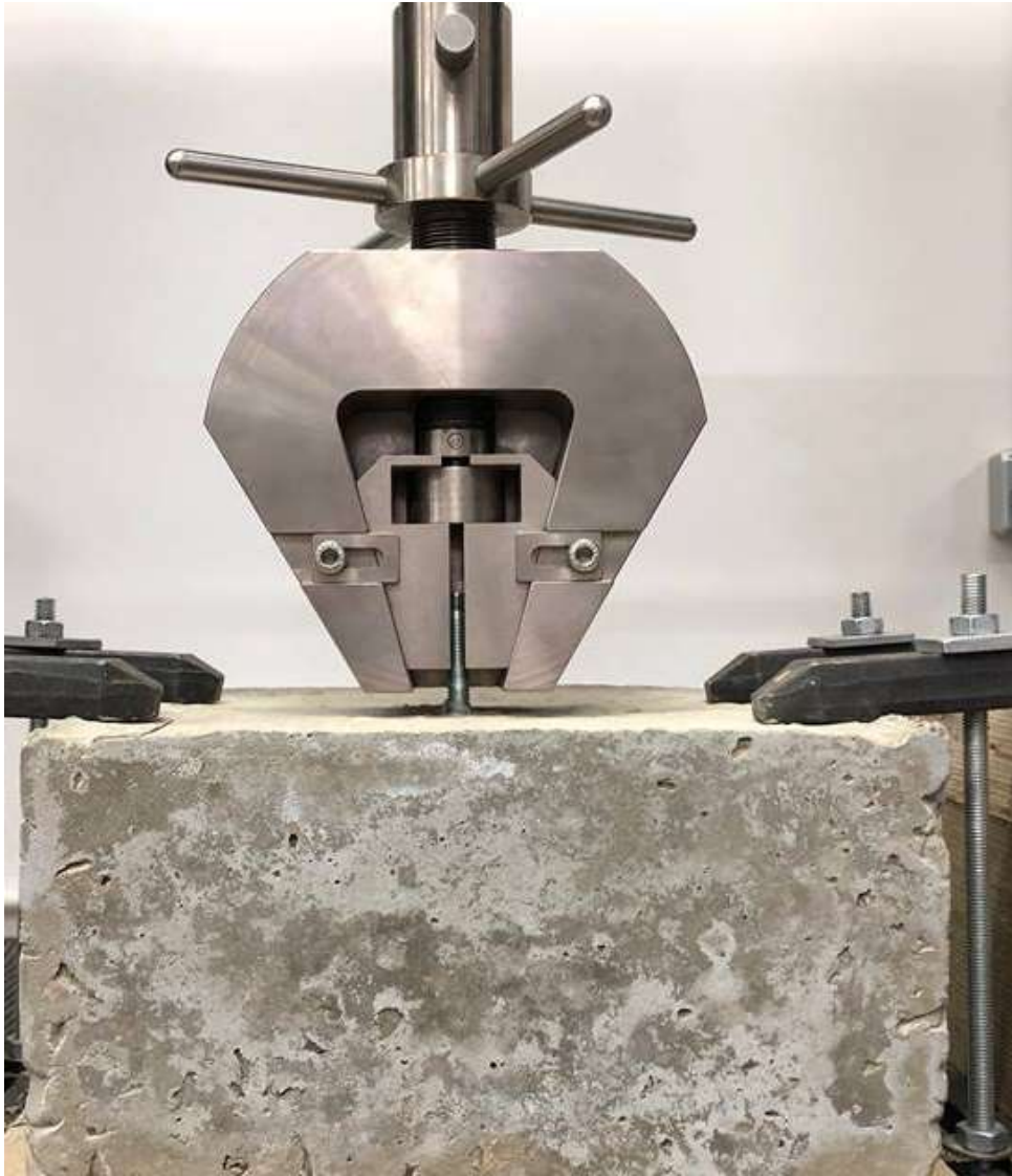
Figure 5 – Bolt pull out details, Lloyds LR100k apparatus
