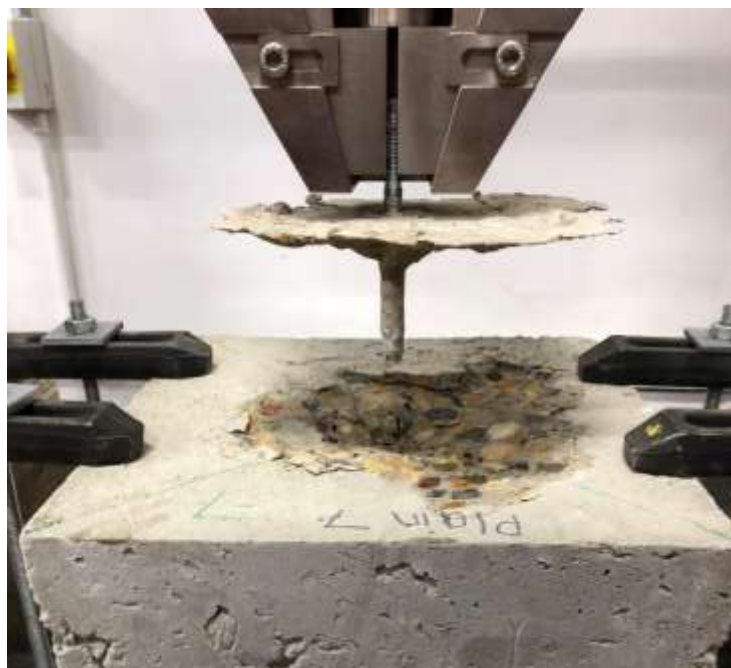
Figure 12: Cone failure of Slab 7
