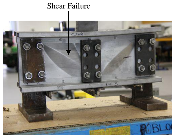
(a) 200x51x1.15x0.95 RHFCB (Test 5, AR of 1.0)
