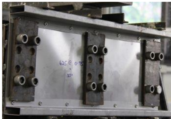
(c) 250x51x1.15x0.95 RHFCB (Test 7, AR of 1.0)
