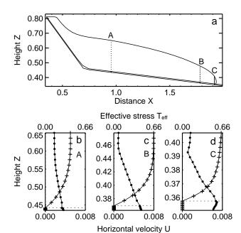
**Fig. 3.** Experiment A: Relatively stiff and moderately non-linear till (m=3, B=8): **(b–d)** vertical profiles of the non-dimensional horizontal velocity U (lines with crosses) and effective stress  $T_{\rm eff}$  (lines with dots) are shown at a dimensionless time T=15.4 for the three locations A, B and C shown in **(a)**. Note that the vertical scale changes for each profile.
