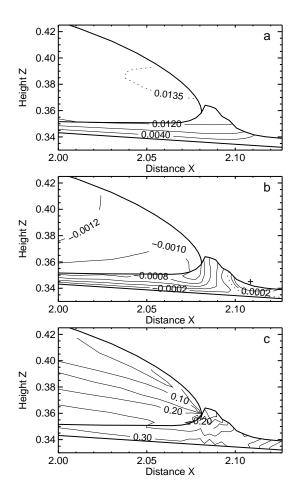
**Fig. 7.** Experiment B: Relatively soft and moderately non-linear till (m=3, B=0.35): Snapshots at dimensionless time T=15 showing the distribution of horizontal velocity (a), vertical velocity (b) and effective stress (c) in the frontal part of the glacier. In (b) the dashed line represents the zero velocity contour line and the symbol + means positive vertical velocities, that is upward movement.
