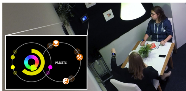
Figure 2. Smart Home Control Demo. Left: clockwise tracking of the moving yellow target increases light intensity (counter clockwise decreases), whilst tracking the purple target navigates through the HUE color spectrum. Right: three room lighting presets.
