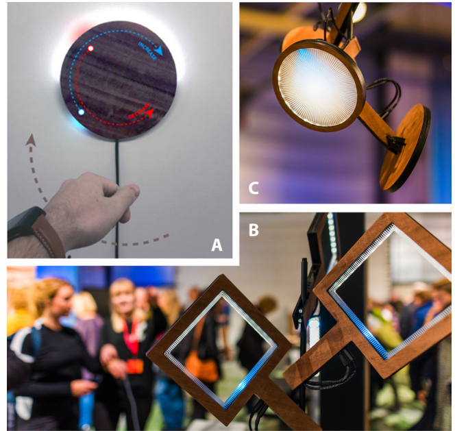
Figure 6. The three proposed interactive lamps: the wall- (A), standing- (B) and ceiling-lamp (C). For the wall-lamp (A), tracking a blue or red LED traversing across the border of the lamp either increases or decreases the amount of light emitted. Photo B and C © Twycer and Mind the Step.
