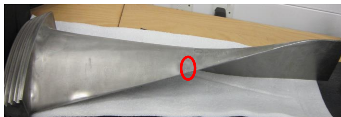
Fig. 13: Steel blade with thermal fatigue natural crack
