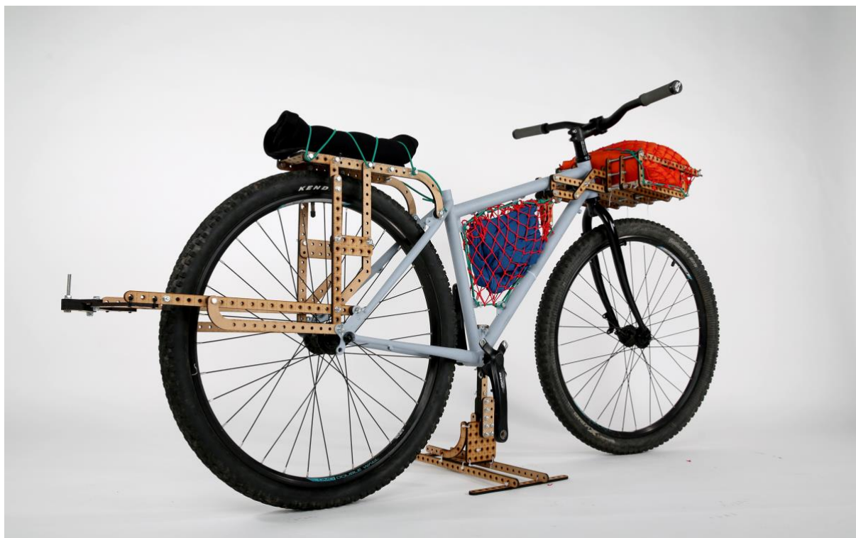
Figure 3: ‘OpenCycle’ prototype produced as part of the collaboration with Organisation 03. A typical bicycle that has been modified to incorporate fixing points located relative to the OpenStructures grid (Lommée, 2012), to create a highly adaptable open-source attachment system.
