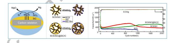
A new hollow nanostructure of sea-sponge-C/SiC@SiC/C has been successfully fabricated by the sea-sponge-C/SiC nanospheres are coated with SiC/C shells through an in situ reduction process, and show an excellent and stable Li<sup>+</sup> storage capability.
